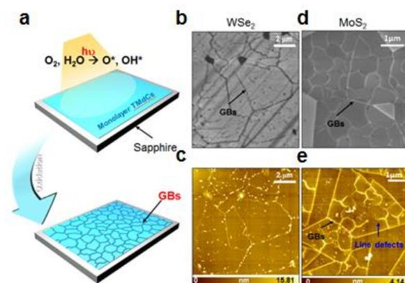
(a) Schematic of the ultraviolet irradiation process. (b,c) SEM and AFM image of oxidized WSe<sub>2</sub>. (d,e) SEM and AFM image of oxidized MoS<sub>2</sub>.
